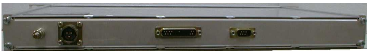
Figure 3 – RIU Rear view (connectors panel)
